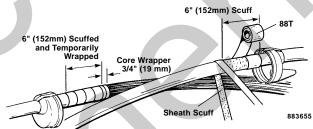
a. Insert base assemblies of shield connectors between the core wrapper and the shield 180 apart.
